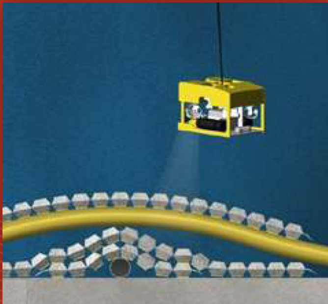
GROUT BAG INSTALLATION
