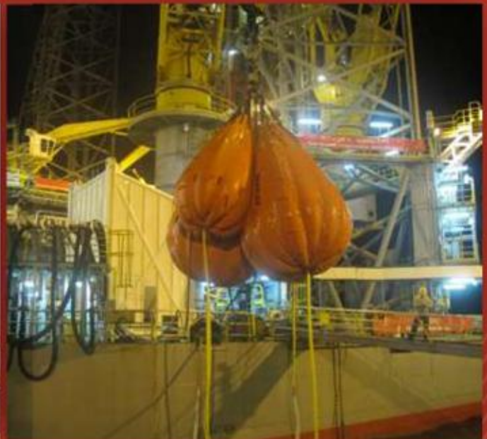
CRANE LOAD TEST JACK UP RIG HYSY 937
