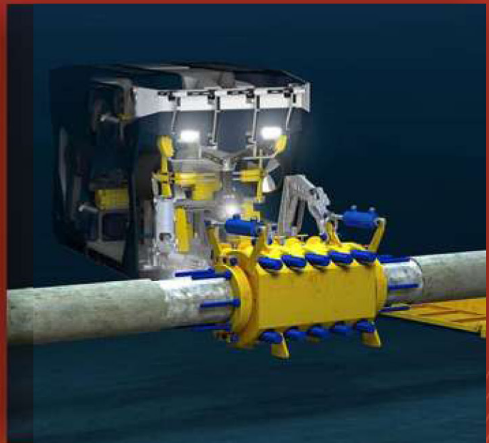
PLIDCO CLAMP INSTALLATION BY ROV WORK CLASS
